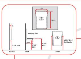
Due to the sleek, vertical design we incorporated a large bed size into a compact, space saving bathroom fixture. This versatile unit is ideal for restrooms where space is of concern because the unit is only 22" wide. When not in use, the closed unit is in compliance with ADA 4.4.1. Protruding Objects when installed to the manufacturer's specifications.
